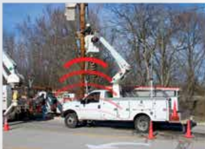
Alerts crews and bystanders when basket is descending with an audible statement, "Warning, aerial lift descending!".
