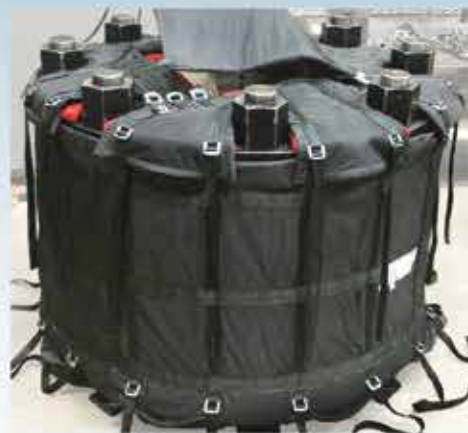
300,000 psi Fracking Test Containment
