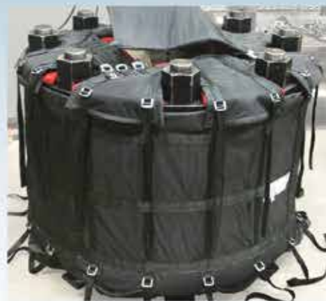
300,000 psi Fracking Test Containment
