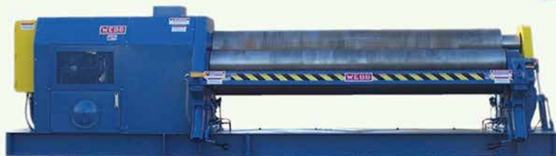
FOUR ROLL HYDRAULIC PLATE ROLL
