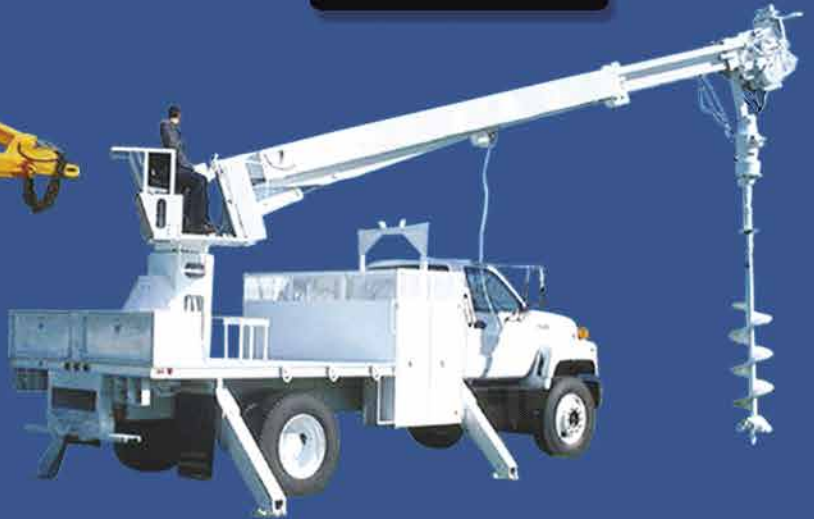
CHEVROLET Diesel Texoma TX-245B Digger Derrick
